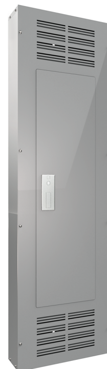
NEMA 1 Enclosure with Vented Hinged Trim Front with 3 Point Latch (required if 175 A or 200 A QO(VH) circuit breakers are installed)
